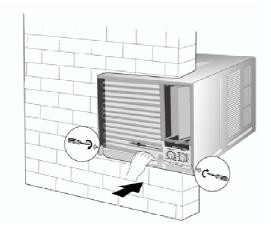
Depending upon the location of the AC outlet, route the AC cord to either the left or right side while installing the front grille.
